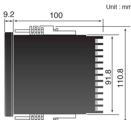
For mounting of the controllers, panel thickness must be between 1 to 10mm. When mounting multiple controllers close together, the panel strength should be checked to ensure proper support..
